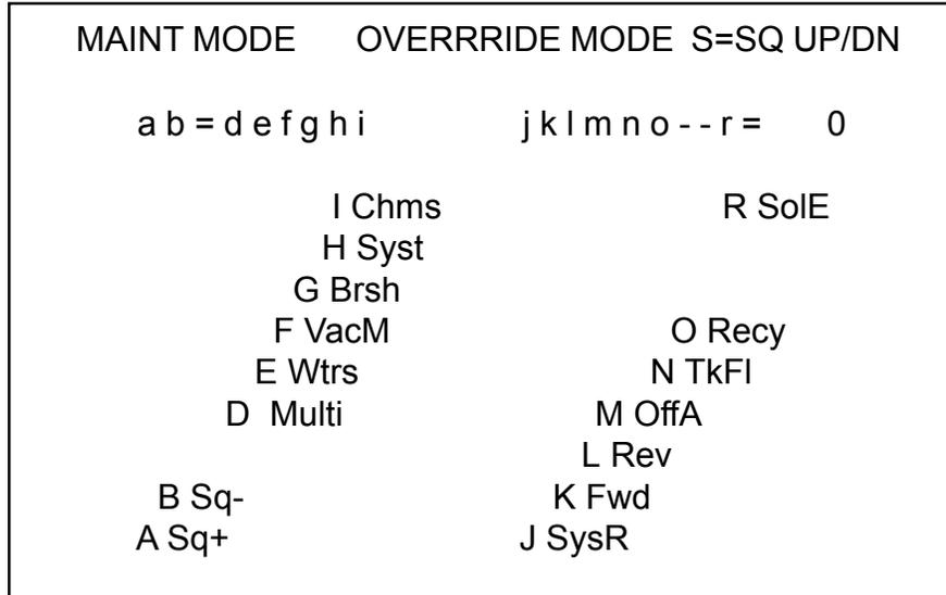
When this screen is active, pressing A,B,D,E,F,G,H,I will change the state of the output relays. To raise/lower the squeegee both the A and B outputs must change. As indicated on the first line, pressing “S” will raise/lower the squeegee (This actually is changing A and B simultaneously).
